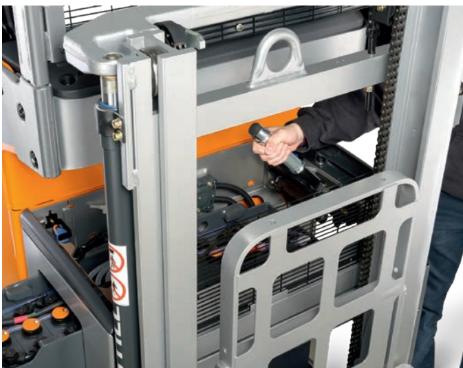
Standard lateral battery change for maximum availability and ergonomics
