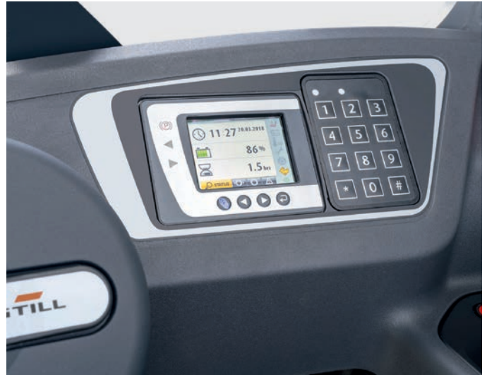
Everything in view, all the time: display shows battery status, date and time
